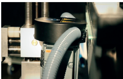
Double grinding wheel with rough (P120) and smooth (P320 or P400) abrasive belt
